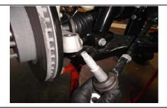
Remove the tie rod ends from the steering knuckle using a 21mm socket.
