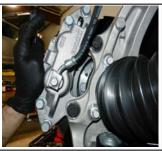
Unbolt the axle nut using a 36mm socket. Use a soft mallet or press tool to knock the axle from the knuckle. Remove the brake calipers from the 7. knuckle using a 18mm socket. Hang out of the way.
