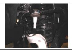
Separate the upper control arm from the steering knuckle using an 18mm socket. **Note:** the upper control arm will be under tension.
