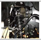
DO NOT over extend the cv-axle joints, doing so will damage/ break them.
