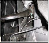
Loosen the upper control arm using a 13/16" socket and wrench. Let it rest on the droop stop, then retighten the upper control arm and torque it down to 90ft lbs. Loosening the lower control arms may be needed as well.
