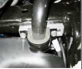
Install the sway bar offset spacers to the frame using the factory 10mm bolts.
