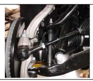
Reinstall the tie-rod using a 21mm socket. Reinstall the sway bar end links 20.
