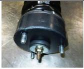
Install the rubber isolator and ReadyLIFT top hat spacer onto the strut using a supplied washer and gold 10mm x 1.5 flange nut. Use a 15mm and 6mm wrench. Make sure to line up the markings from top to bottom on the 15. strut. Do not use an impact gun, tighten down by hand.
