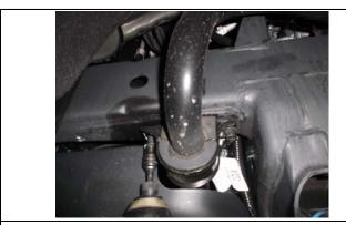
3. Loosen the factory sway bar at the frame using a 10mm socket.
