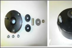
Install the rubber bushings to each side of the spacer. Lube the metal 14. sleeve and press into the bushings.
