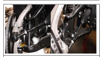
Remove the sway bar end links from the vehicle. Using a 15mm socket on top and a 13 mm socket on bottom.
